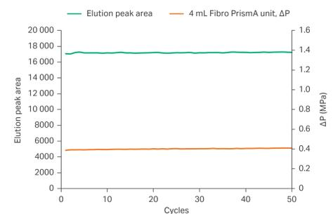
**Fig 4.** Trend curves of max delta column pressure ( $\Delta P$ ) and area of elution peak performance over cycles.
