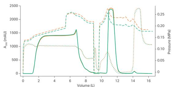
**Fig 7.** Overlaid chromatograms: cycles 1 and 13 of Fibro PrismA prototype 600 mL unit.
