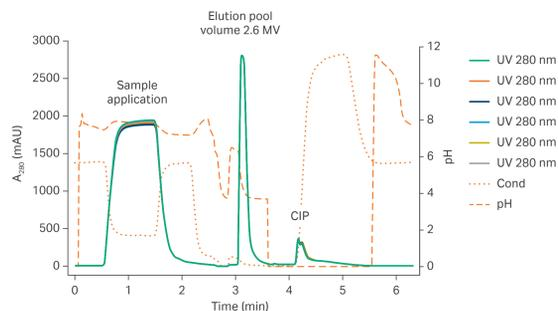
**Fig 3.** Protein A bind-elute profile on clarified cell culture mAb feed of 3.8 mg/mL purified on a ~4 mL Fibro PrismA unit: Overlay UV<sub>280</sub> nm every 10th cycle, cycle time 6.3 min, flow rate 8 MV (CIP 4 MV).
