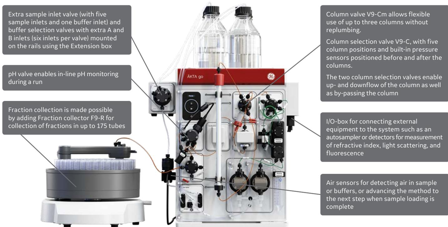
Fig 4. Optional components can be added in the two empty positions in the system chassis or mounted on rails to expand the capability of the ÄKTA go system. A total of maximum six options can be added at the same time.
