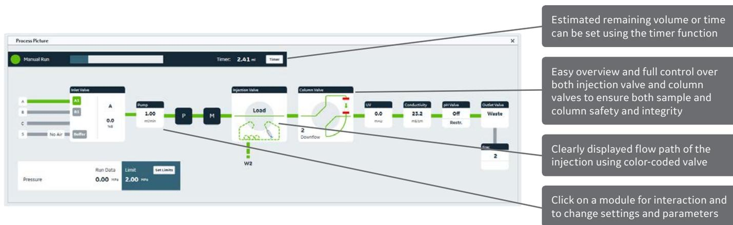
**Fig 7.** The **Process picture** represents the system flow path with a clear overview of placement of system components. All parts of the system are interactive and developed to ensure integrity of your run, samples, and columns.
