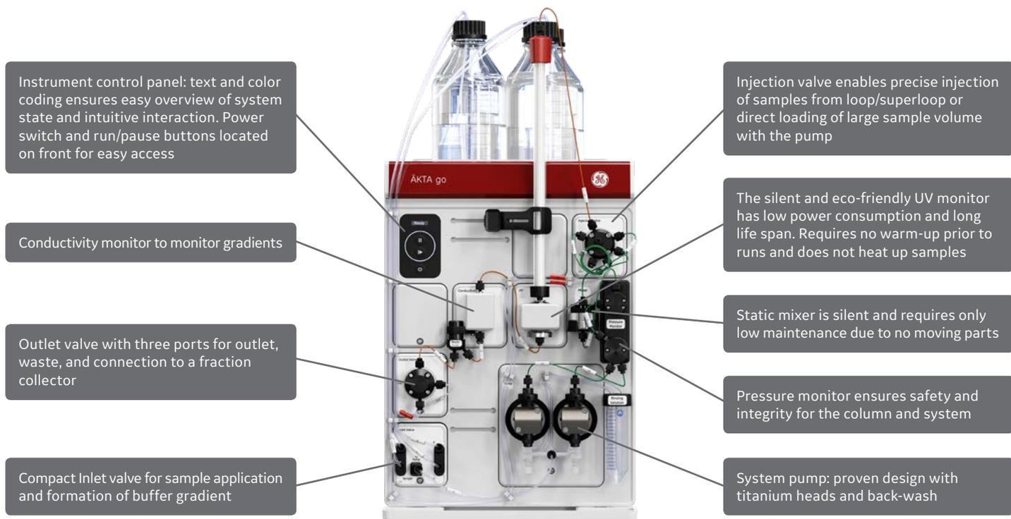
Fig 3. ÄKTA go standard system and its components.
