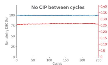
**Fig 5.** DBC performance of protein A Fibro unit over 250 cycles. Sample: clarified cell culture fluid with a mAb titer of 3.8 mg/mL, with no cleaning in place (CIP) carried out between runs. A flow rate of 15 mL/min was used for all phases on a 0.2 mL adsorbent volume, 2 min/cycle, to a 30 mg/mL load challenge.
