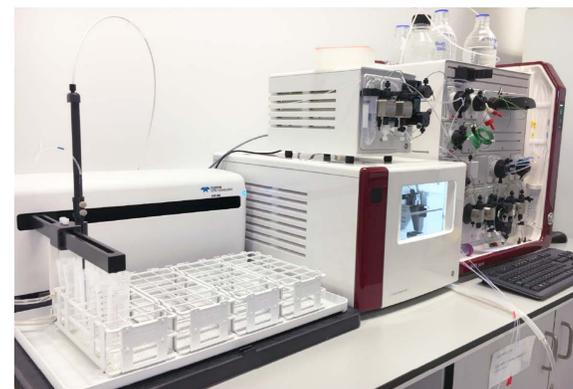
**Fig 6.** This picture illustrates a set-up facilitating high-throughput purification using the autosampler ASX-560 (left), sample pump (middle top), fraction collector (middle bottom), and ÄKTA pure 25 system (right).
