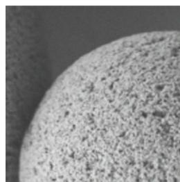
**Fig 1.** Conventional chromatography: diffusive flow. Mass transfer is restricted by the slow diffusion of molecules through the pores of the bead, and process flow is restricted by the rigidity of the beads.
