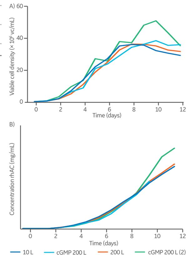
**Fig 4.** (A) Viable cell density and (B) cell productivity over the culture period for the selected clone (47) cultured in XDR-10 and XDR-200 bioreactor systems.
