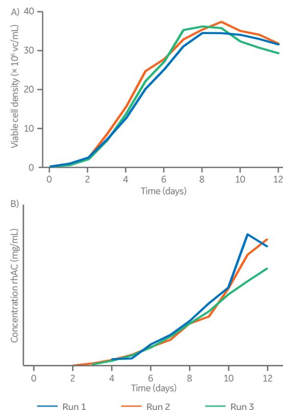
**Fig 3.** (A) Viable cell density and (B) cell productivity over the culture period for the selected clone (47) cultured in XDR-10 bioreactor system.
