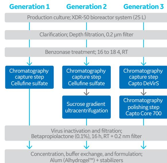
**Fig 7.** The initial virus production process, including purification on Cellufine sulfate resin, was complemented with an ultrafiltration step to improve HCP reduction. In the final optimized process, Cellufine sulfate and ultracentrifugation steps were replaced by two chromatography steps based on Capto resins.
