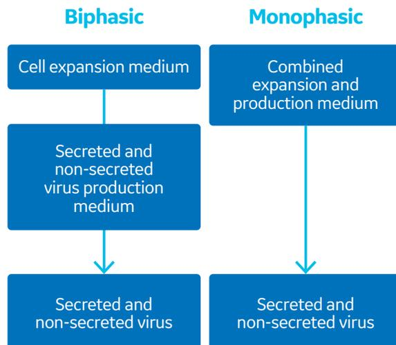
**Fig 4.** While traditional virus production in EB66 cells is biphasic, requiring two or more media and multiple additives, CDM4Avian medium is designed to support the simpler monophasic approach, requiring fewer additives.
