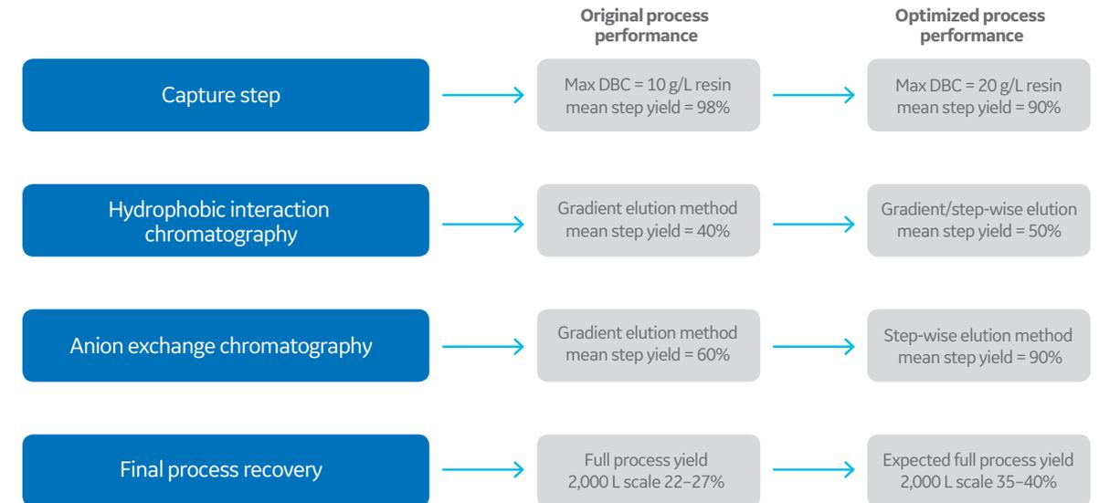
**Fig 4.** Improvements from the original process, using the optimized process
