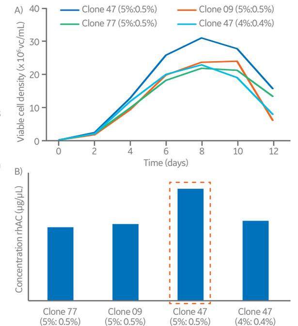
**Fig 1.** (A) Viable cell density over the culture period and (B) cell productivity on Day 12 of the tested clones in shake-flask cultures.
