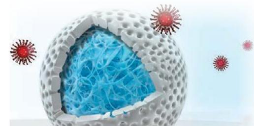
**Fig 5.** Schematic representation of Capto Core 700 shows a bead with the inactive, porous shell and the ligand-containing core. Proteins and impurities penetrate the core, while target viruses and larger biomolecules ( $>M_r$  700,000) are excluded from the resin and pass in the flowthrough.
