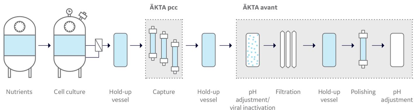
**Fig 1.** Schematic overview of the connected and integrated process, with hold-up vessels placed between the different unit operations.
