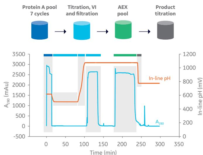
**Fig 2.** Schematic chromatogram, showing UV and pH from the different unit operations. Once 21 elution fractions from ÄKTA pcc were collected, a signal was sent to ÄKTA avant to start the pH adjustment for viral inactivation (VI). After VI, the pH was adjusted again, after which the material was filtered. The filtrate was applied to an AEX column, and the mAb-containing flowthrough was finally titrated to a pH suitable for the mAb (2).
