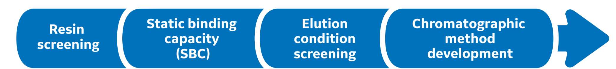
Fig 1. The standardized workflow applied for evaluating and selecting resins for a polishing step of a biosimilar molecule. The first part consists of screening of a wide area of conditions in a format that allows increased throughput and provides process understanding. The final part involves development of a chromatographic method to identify running conditions in an "easy-to-scale-up" approach.
