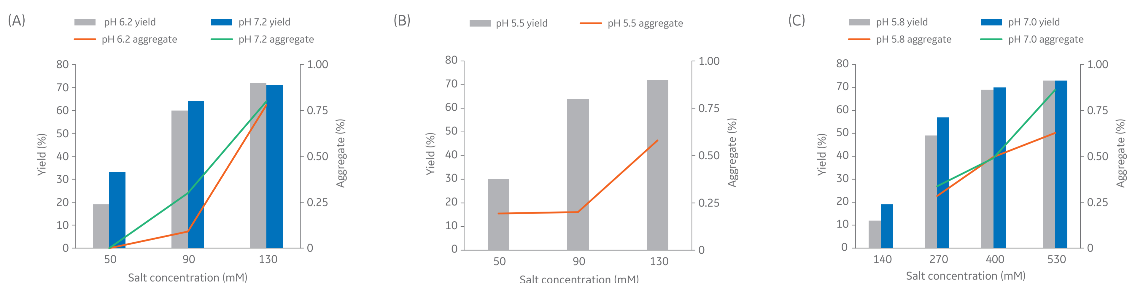
Fig 3. Yield (bars) and aggregate content (lines) for (A) Capto S ImpAct; (B) Capto SP ImpRes; (C) Capto MMC ImpRes.
