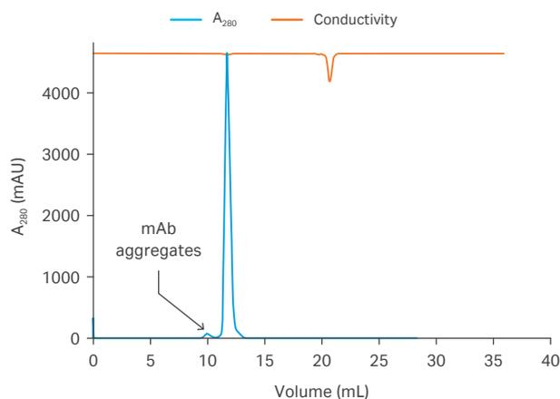
**Fig 5.** (A) Chromatogram from an analytical separation of mAb monomers from aggregates on a 1 mL HiTrap MabSelect Prisma column. (B) SEC analysis of collected fractions on a Superdex 200 Increase 10/300 GL column. By combining the antibody affinity step with high-resolution SEC, an understanding of the antibody profile can be obtained, which is important in the purification process.
