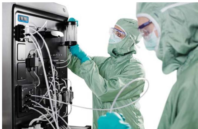
**Fig 1.** The ÄKTA pilot 600 chromatography system is designed to simplify the sanitization procedure, supporting biomanufacturers in meeting the high purity standards imposed by regulatory authorities for clinical products.
