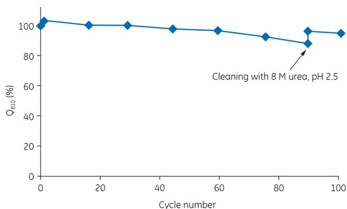
**Fig 15.** The Capto L resin retains more than 90% of its initial binding capacity over 80 cycles with the recommended 15 mM NaOH CIP solution. At cycle 89, the Capto L column was cleaned with 8 M urea at pH 2.5 with positive effects on binding capacity.
