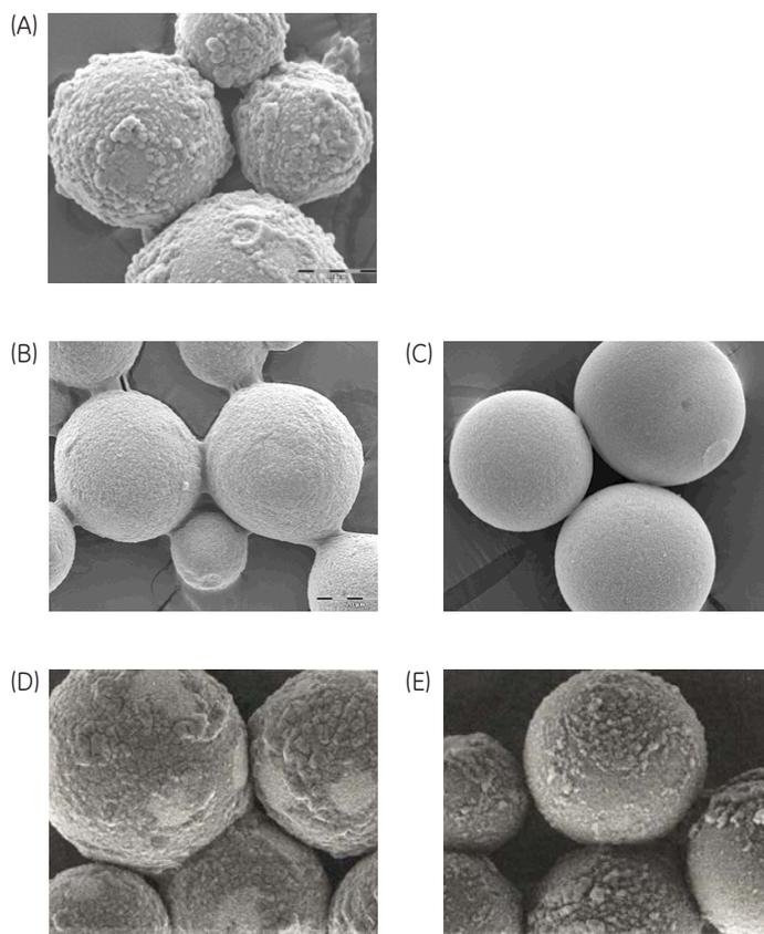
**Fig 4.** (A) Fouling of MabSelect particles due to inefficient cleaning with 0.1 M phosphoric acid for 300 cycles in a mAb process. Cleaning with 0.1 M NaOH for (B) 40 min and (C) up to 3 h removed the fouled proteins. Incubation of the fouled particles in 6 M guanidine hydrochloride for (D) 40 min or (E) 3 h did not offer the same cleaning effect as 0.1 M NaOH. Reprinted with kind permission from Genentech, CA, USA.
