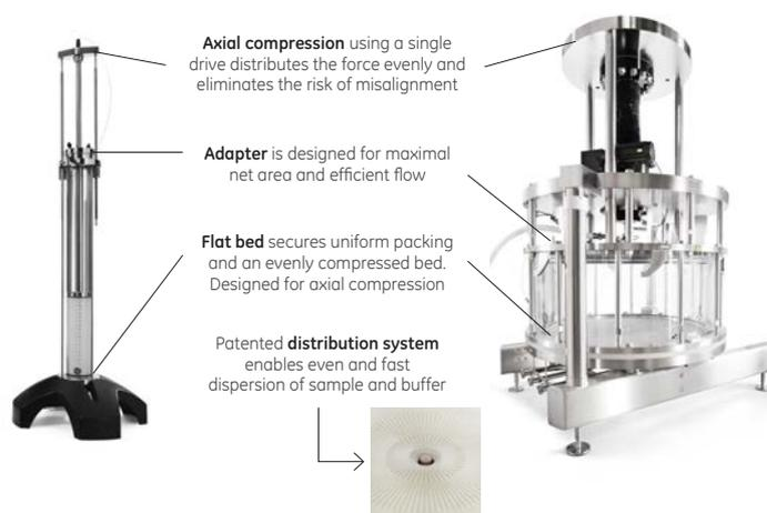
**Fig 2.** The AxiChrom™ column design allows for automated packing and unpacking of the column. The column design also enables cleaning with the adaptor raised, by flowing the cleaning liquid upwards through a liquified bed in a closed manner (9). The fluidized bed can thereafter be repacked without opening the column.
