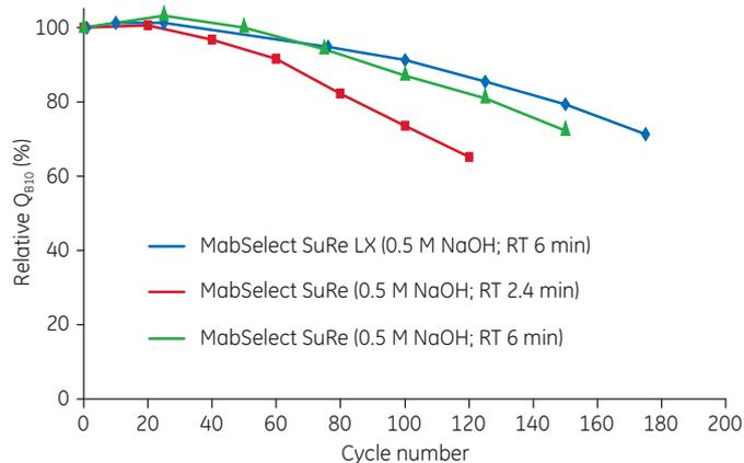
**Fig 10.** Remaining DBC at 10% breakthrough ( $Q_{B10}$ ) of MabSelect SuRe and MabSelect SuRe LX resins after CIP with 0.5 M NaOH for 0–175 cycles. DBC was tested using polyclonal IgG and residence times of 2.4 and 6 min.
