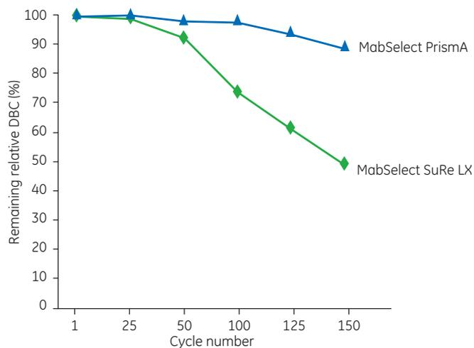
**Fig 13.** Cycling of MabSelect Prisma and MabSelect SuRe LX using pure buffers and 1.0 M NaOH for cleaning in each cycle shows that MabSelect Prisma maintains > 90% of its initial capacity after 150 cleaning cycles.
