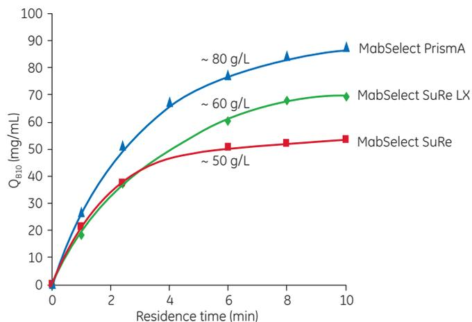
**Fig 12.** Compared with MabSelect SuRe LX, the optimized base matrix of MabSelect Prisma offers an up to 40% increase in DBC at a residence time of 2.4 min or a 30% increase in DBC at 4 min residence time. At 6 min residence time, a binding capacity of 80 mg human IgG/mL resin was observed for MabSelect Prisma, which is more than 25% higher than for MabSelect SuRe LX.
