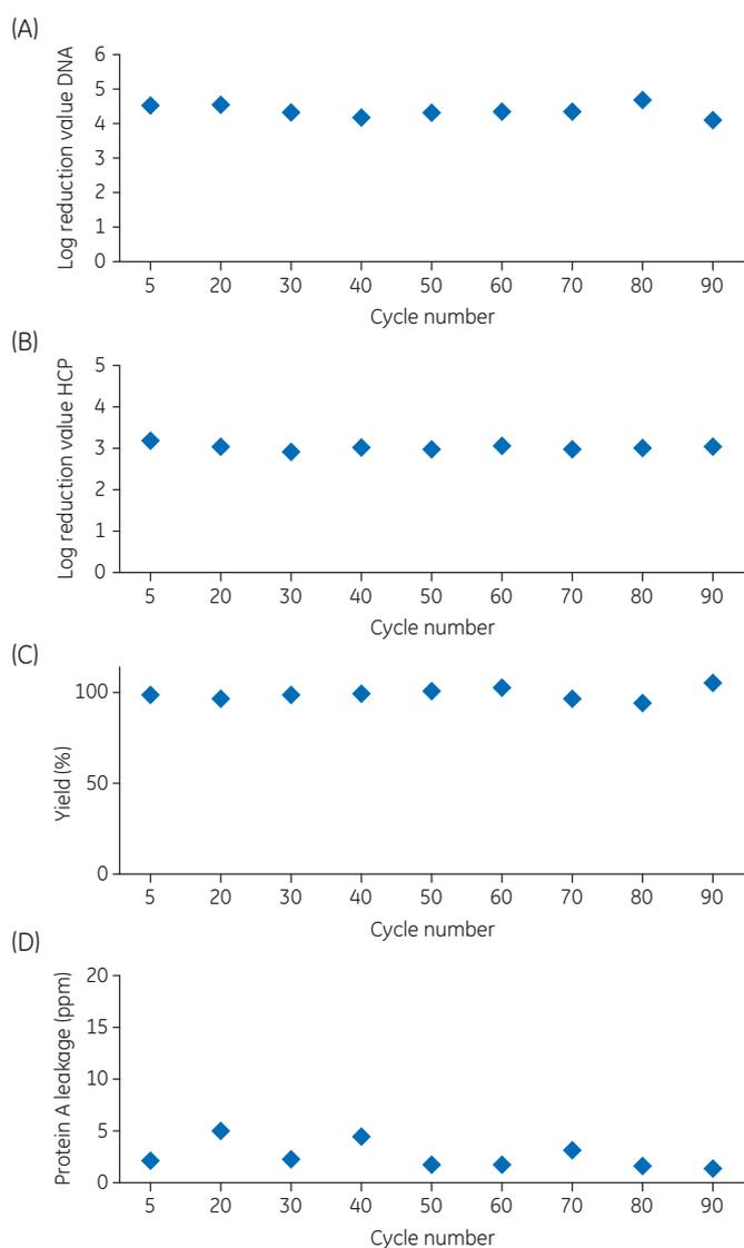
**Fig 11.** MabSelect SuRe LX exhibits stable (A) hcDNA clearance, (B) HCP clearance, and (C) mAb yield as well as (D) low ligand leaching using 0.5 M NaOH for cleaning at a contact time of 15 min over 90 cycles.
