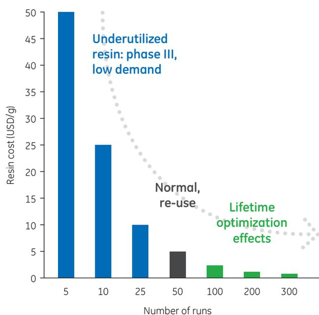
**Fig 1.** Process economy effect of resin reuse. The calculation is based on a 300 L protein A column, 10 kUSD/L, 40 g/L capacity. Adapted from "Biopharmaceutical processing: development, design, and implementation of manufacturing processes" with kind permission of Elsevier, Amsterdam, NL. (2).
