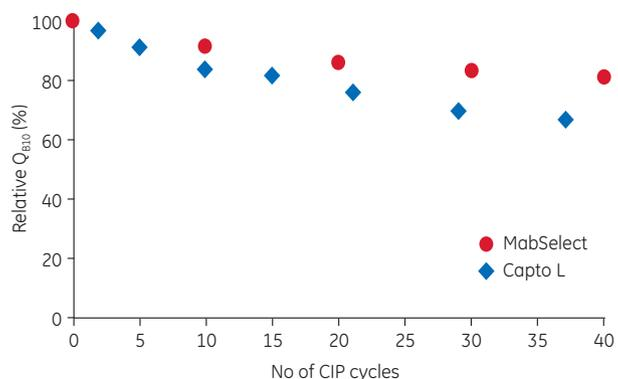
**Fig 7.** Remaining DBC at 10% breakthrough ( $Q_{B10}$ ) of MabSelect and Capto L resins. The stability of Capto L under caustic conditions was investigated and compared with that of MabSelect resin. The resins were both exposed to repeated CIP cycles using 0.1 M NaOH at a contact time of 15 min.
