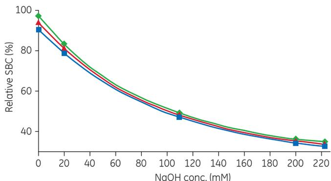
**Fig 8.** PreDictor plates were used for screening of resin compatibility in NaOH. Remaining static binding capacity (SBC) of MabSelect resin after storage in 0–220 mM NaOH for 43 h, corresponding to 172 CIP cycles at 15 min contact time. The remaining capacity decreases with increasing NaOH concentration. For a remaining capacity of > 80%, NaOH concentration needs to be below 20 mM.
