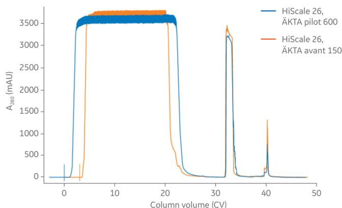
**Fig 2.** Overlay of chromatograms from mAb capture on the HiScale 26 column using ÄKTA avant 150 and ÄKTA pilot 600. The two curves are aligned from the start of elution. Feed concentrations were 3.5 mg/mL for the ÄKTA avant 150 process and 2.7 mg/mL for the ÄKTA pilot 600 process.
