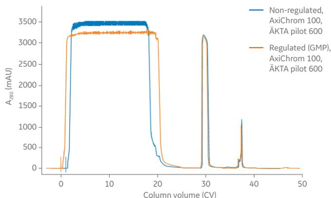
**Fig 4.** Overlay of chromatograms from mAb capture on AxiChrom 100 using ÄKTA pilot 600 in a non-regulated (non-GMP) and regulated (GMP) environment. Feed concentrations were 3.5 mg/mL for the non-regulated process and 3.0 mg/mL for the regulated process.
