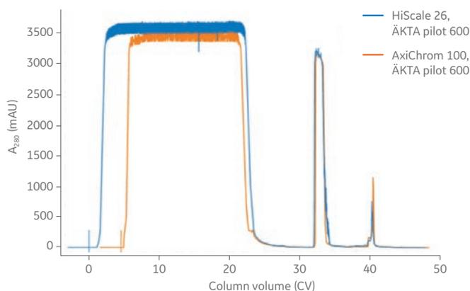
**Fig 3.** Overlay of chromatograms from mAb capture on the HiScale 26 and AxiChrom 100 columns, both operated on ÄKTA pilot 600. Feed concentrations were 2.7 mg/mL for the HiScale 26 column and 3.0 mg/mL for the AxiChrom 100 column.
