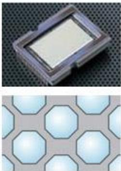
\* 1 large CCD: "Super CCD", 320 million octagonal shaped pixels of the light-detecting elements are placed at a diagonal angle. The pixel size per unit area of this CCD is larger than conventional CCD and it has achieved the same level of high sensitivity with X-ray film. In addition, the image data is output at high resolution of up to 6.3 million pixels by unique technology developed by Fujifilm. This enables the imager to achieve both high sensitivity and high resolution.
