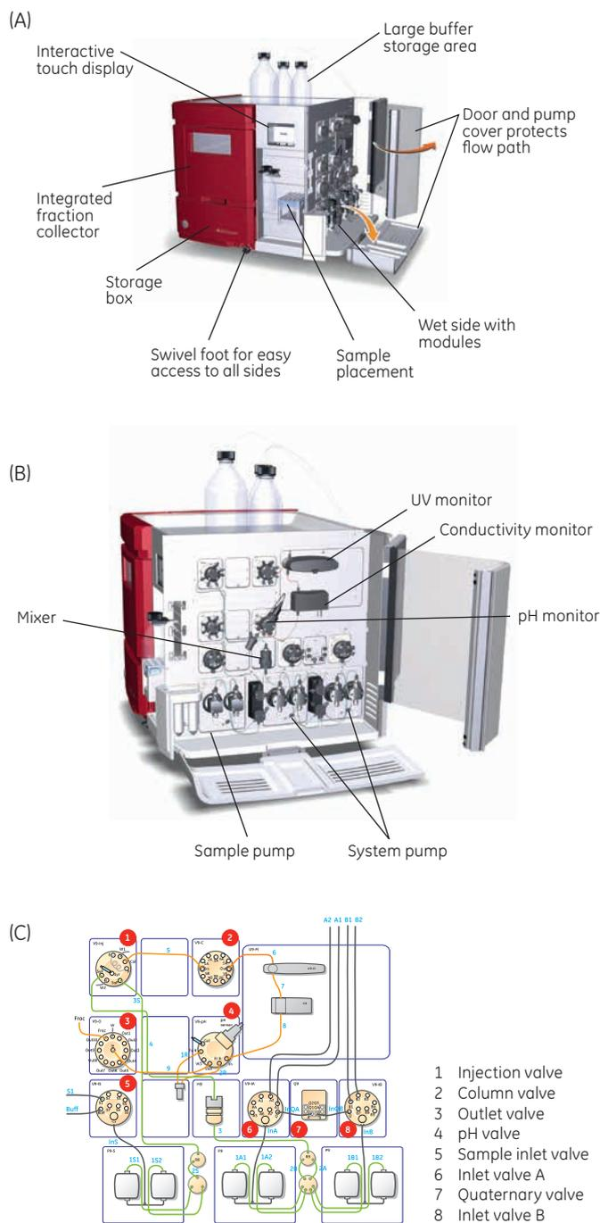
**Fig 2.** (A) Features of ÄKTA avant; (B) an illustration of the wet side; (C) a diagram showing the wet side.
