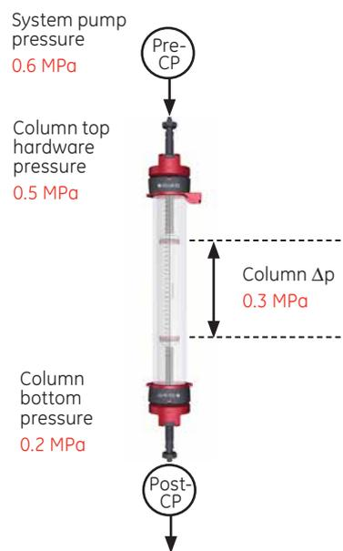
**Fig 3.** For increased operational safety, the column selection valve enables continuous measurement of precolumn (Pre-CP) and post-column pressure (Post-CP) during runs. The pressure difference over the packed medium bed ( $\Delta p$ ) is calculated from the two signals.
