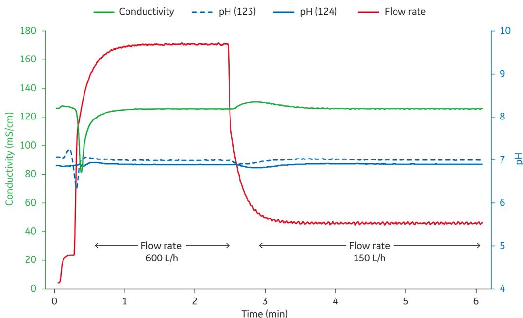
**Fig 4.** Preparation of 10 mM Tris buffer, 1 M  $(\text{NH}_4)_2\text{SO}_4$ , pH 7.0 from the stock solutions 0.1 M Tris-HCl, 0.01 M Tris base, and 3 M  $(\text{NH}_4)_2\text{SO}_4$  at 600 and 150 L/h using pH-Flow feedback. Preparation time was 1.0 min for both flow rates.
