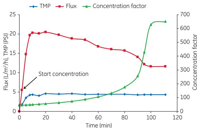
**Fig 6.** Step 2 sample concentration from 2 to 0.1 L.
