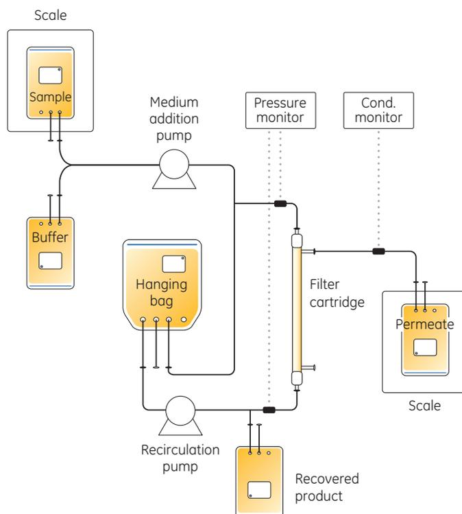
**Fig 1.** Schematic drawing of the filtration setup.
