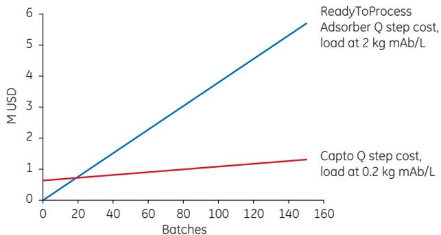
**Fig 5.** Accumulated mAb manufacturing costs for the final polishing step (2000 L process scale). For Capto Q, costs for labor, buffer/process liquids, resin, column hardware, resin packing and lifetime study, as well as cleaning and storage of the packed column are included. For ReadyToProcess Adsorber Q, costs for membrane, labor, and buffer/process liquids are included.
