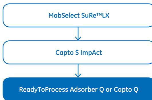
**Fig 1.** Classical three-step mAb purification process, using MabSelect SuRe LX protein A resin for capture, Capto S ImpAct cation exchange resin for intermediate purification, and either ReadyToProcess Adsorber Q membrane or Capto Q resin for final polishing by anion exchange chromatography.
