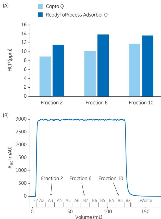
**Fig 3.** (A) HCP content in selected fractions from the column verification experiments (amount of HCP at start was 180 ppm). (B) Chromatogram from the ReadyToProcess Adsorber Q run, showing fractions analyzed for HCP content (the Capto Q run resulted in a similar chromatogram).
