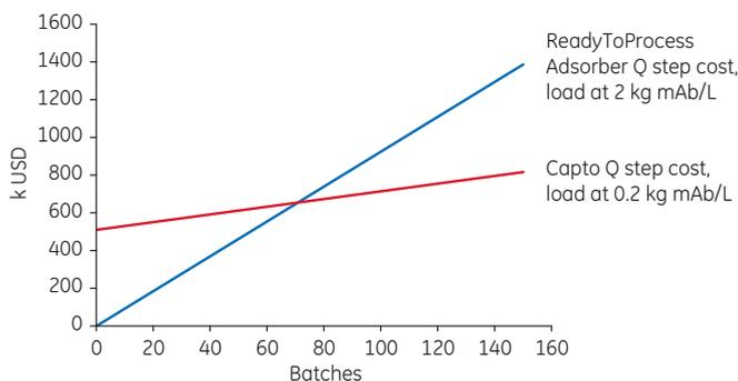
**Fig 4.** Accumulated mAb manufacturing costs for the final polishing step (500 L process scale). For Capto Q, costs for labor, buffer/process liquids, resin, column hardware, resin packing and lifetime study, as well as cleaning and storage of the packed column are included. For ReadyToProcess Adsorber Q, costs for membrane, labor, and buffer/process liquids are included.
