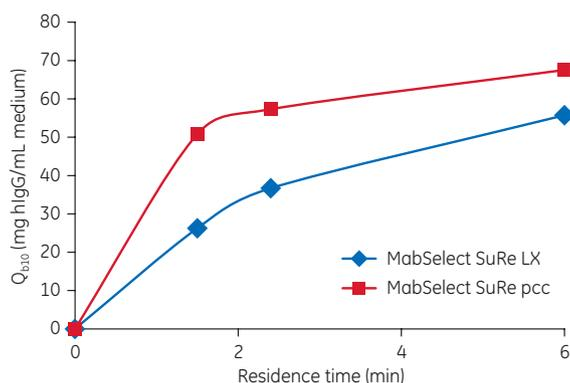
**Fig 2.** DBC at 10% breakthrough ( $Q_{b10}$ ) for a human polyclonal IgG antibody (hIgG) as a function of residence time.
