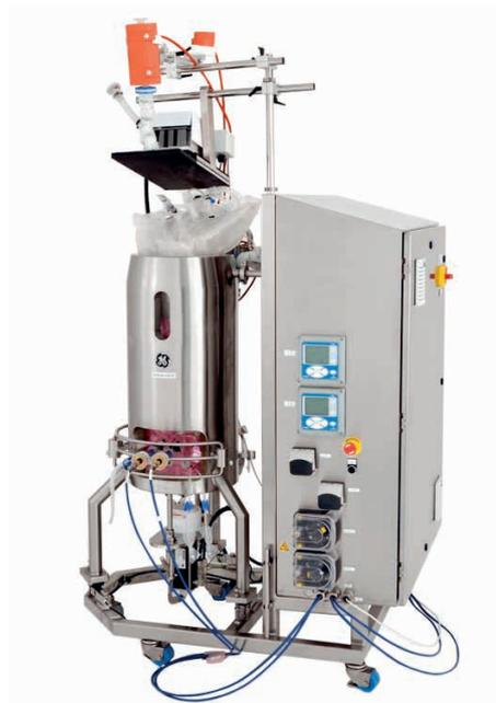
Fig 1. XDR-50 MO fermentor vessel and I/O cabinet.
