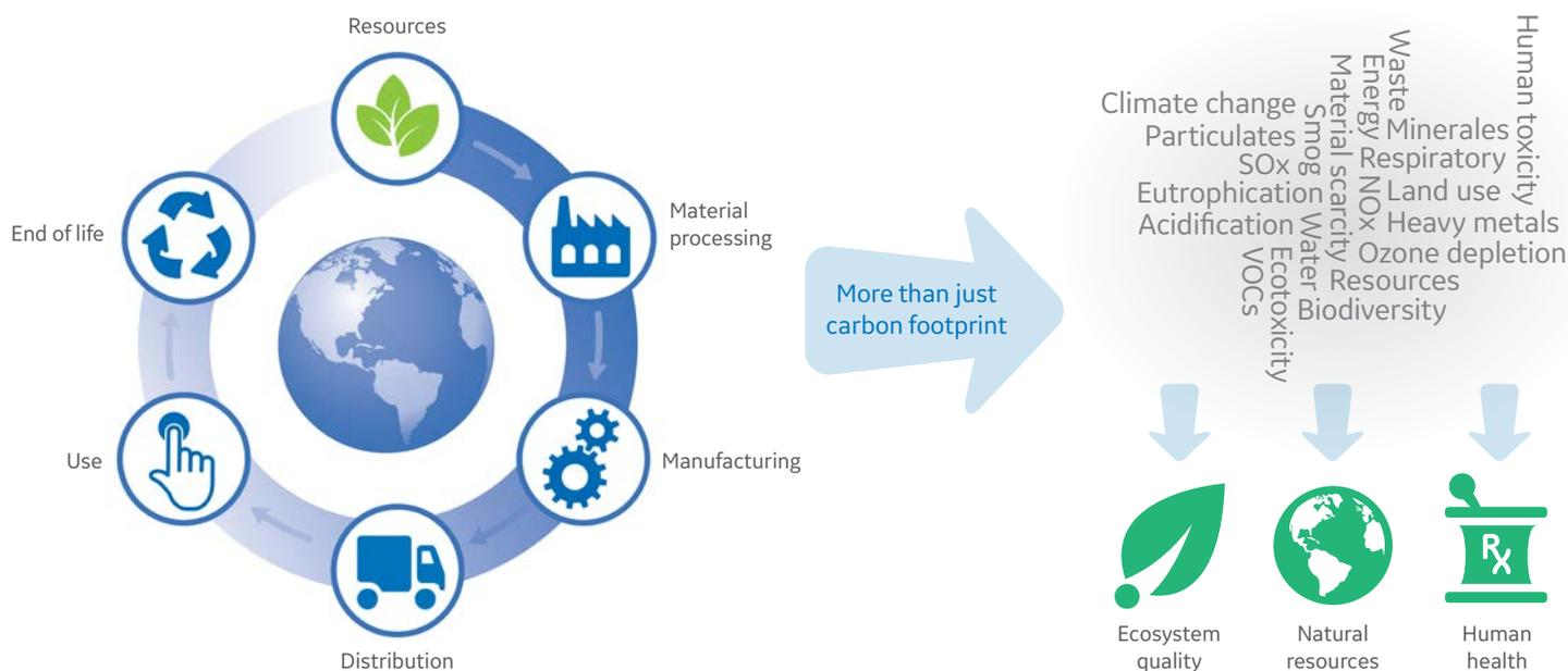
**Fig 1.** Schematic diagram of the product life cycle (left) and impacts evaluated in Life Cycle Assessment (LCA). LCA is a powerful approach that allows one to evaluate environmental impacts, benefits, trade-offs, and burden shifts across the product life cycle, from cradle-to-grave.
