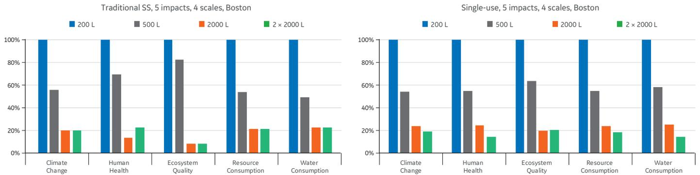
**Fig 4.** Impact comparison for traditional and single-use process technologies at four process scales, from 200 L to 2 x 2000 L mAb production. Location is Boston, USA, and end-of-life disposal is autoclaved followed by landfill.
