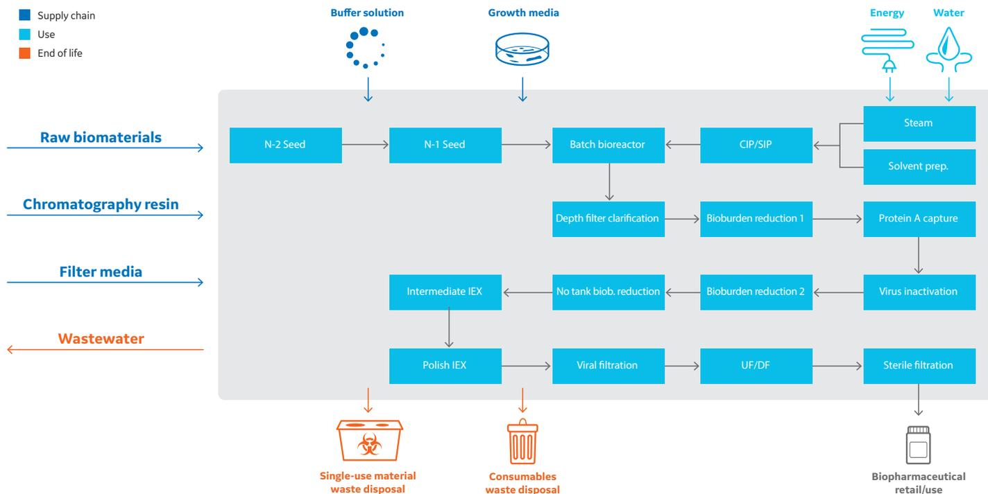
**Fig 2.** mAb bioprocessing configuration used in current study. Biob. = bioburden, CIP/SIP = cleaning/sanitization in place, IEX = ion exchange chromatography, Prep. = preparation, UF/DF = ultrafiltration/diafiltration. Note: General unit operations shown; configuration can change due to scale, product choice, technologies used, etc.
