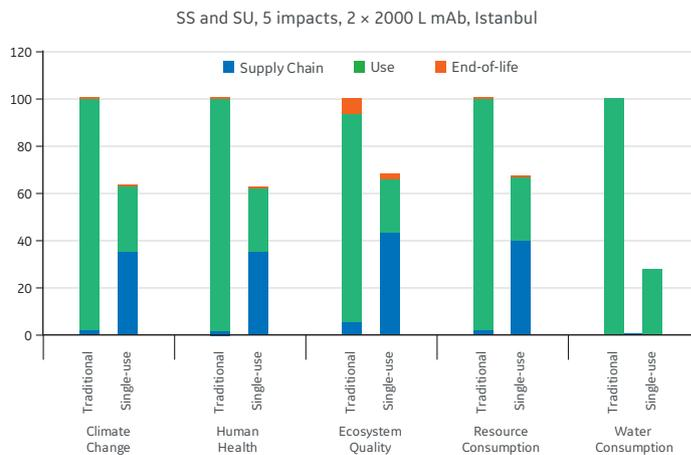
**Fig 3.** Impact comparison for traditional and single-use process technologies. Data are for a 2 × 2000 L scale mAb process located in Istanbul, Turkey. End-of-life disposal is autoclaved followed by landfill.
