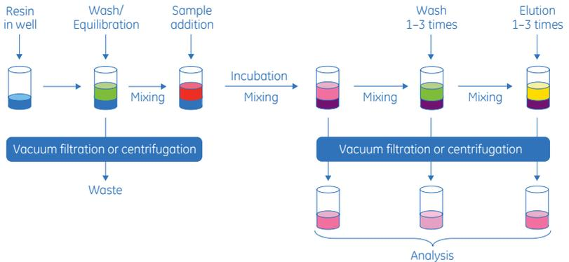
Figure 2.1: Schematic drawing of a batch uptake experiment taking place in the wells of PreDicator plates.
