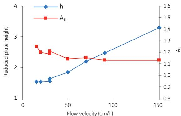
**Fig 6.** The reduced plate height and asymmetry values at different flow rates run on a 20 cm bed of Capto MMC in a BPG 300 column. The curves follow the van Deemter theory showing that the bed is well-packed.
