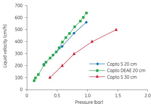
**Fig 6.** Pressure-flow curve in water at 20°C for Capto S and Capto DEAE, 20 cm packed bed height and Capto S 30 cm packed bed height in Chromaflow 600. As the optimal compression factor is difficult to achieve in standard pack-in-place columns, the maximum flow velocity that can be run through the packed bed is limited. The highest operating velocity recommended for this type of column is 500 cm/h compared with in AxiChrom columns where 700 cm/h could be used for a 20 cm bed.
