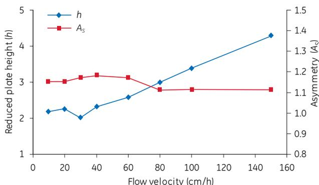
**Fig 7.** The reduced plate height and asymmetry values at different liquid velocities run on a 20 cm bed of Capto S in a BPG 100 column. This is an example, but similar behavior can be expected for packed beds in other columns such as AxiChrom and Chromaflow columns.
