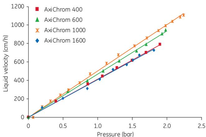
**Fig 3.** Pressure-flow curve in water at 20°C for Capto S, 20 cm packed bed height, in different AxiChrom columns. Capto resins can be run at 700 cm/h with a back pressure of less than 3 bar. System/tubing pressure is excluded.
