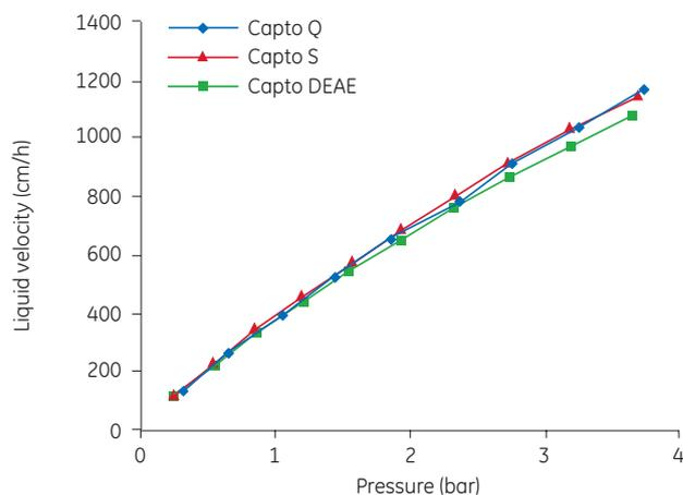
**Fig 4.** Pressure-flow curve in water at 20°C for Capto Q, Capto S, and Capto DEAE, 20 cm packed bed height, in BPG 100. The three resins have nearly the same pressure-flow properties. System/tubing pressure is excluded.
