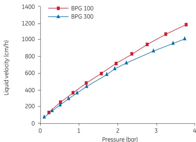
**Fig 5.** Pressure-flow curve in water at 20°C for Capto DEAE, 20 cm packed bed height in BPG 100 and BPG 300, showing that the resin can be run at 700 cm/h with a back pressure of less than 3 bar. System/tubing pressure is excluded.
